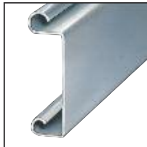
No. 17 — Flat-faced slat in 20 or 22-gauge steel or stainless steel Depth of crown: 1/2", 1/4" on centers.
