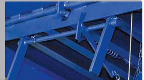
The Blue Giant **C-Series mechanical dock leveler** is easy to operate. Simply pull the release chain- the heavy-duty lift springs raise the deck, and the lip powers out smoothly to the locked position. Then 'walk' the dock down onto the trailer bed. When the truck leaves the loading dock, the lip releases, allowing the unit to be returned to the cross-traffic position.
