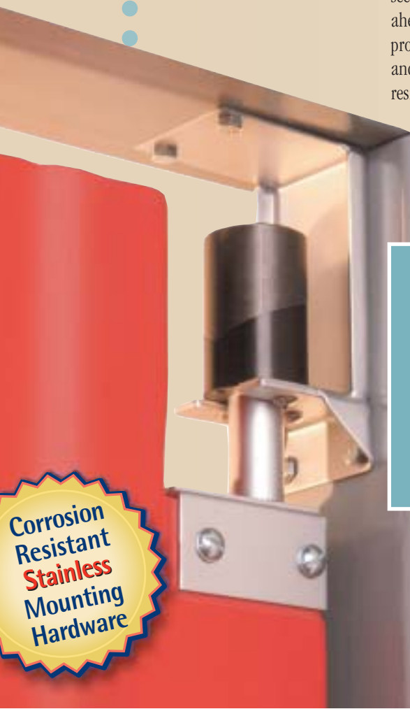
The aluminum upper helix hinge section "climbs" the dark polymer cam section to swing and raise the door without pressure points or edges.
