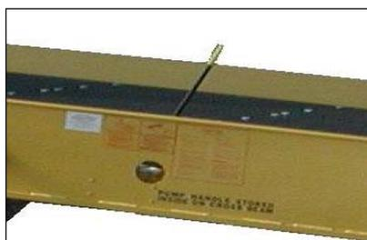
**Pump**—Hydraulic hand pump quickly adjusts top end of ramp with the bed of the vehicle or loading dock. The handle is stored out of the way when not in use.
