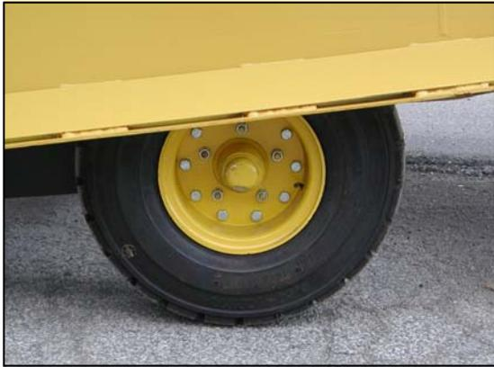
**Pneumatic Tires**— (Standard on all ramps) Premium 23" tires, ideal for use in most applications. Air inflated tires create a cushion effect on irregular or bumpy surfaces. **Solid Filled Tires**- (Option on all ramps) Ideal in applications where sharp debris could puncture a pneumatic tire.
