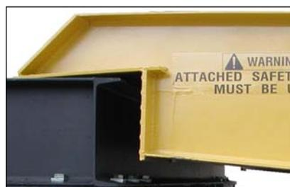
**15" Lip**—Deep overlap of frame at high end is assurance that the ramp rests firmly on the carrier body or dock floor. Eight foot long safety chains and hooks are provided for added security. When correctly rigged, chains join the ramp and vehicle into a single unit.
